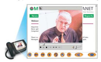
For example, a call from a door entry phone could trigger the picture from an adjacent video or web camera to be displayed on the screen of the PCS 400.
